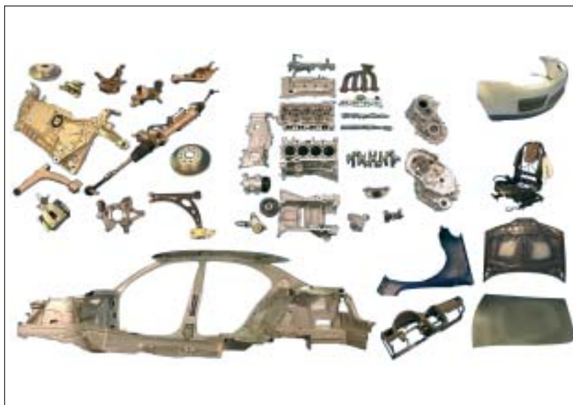
Design analysis of vehicles by entirely tearing them down
