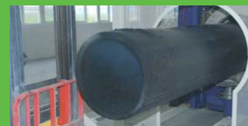
Pipe produced using Hostalen CRP 100 black resins at Krauss Maffei open house
