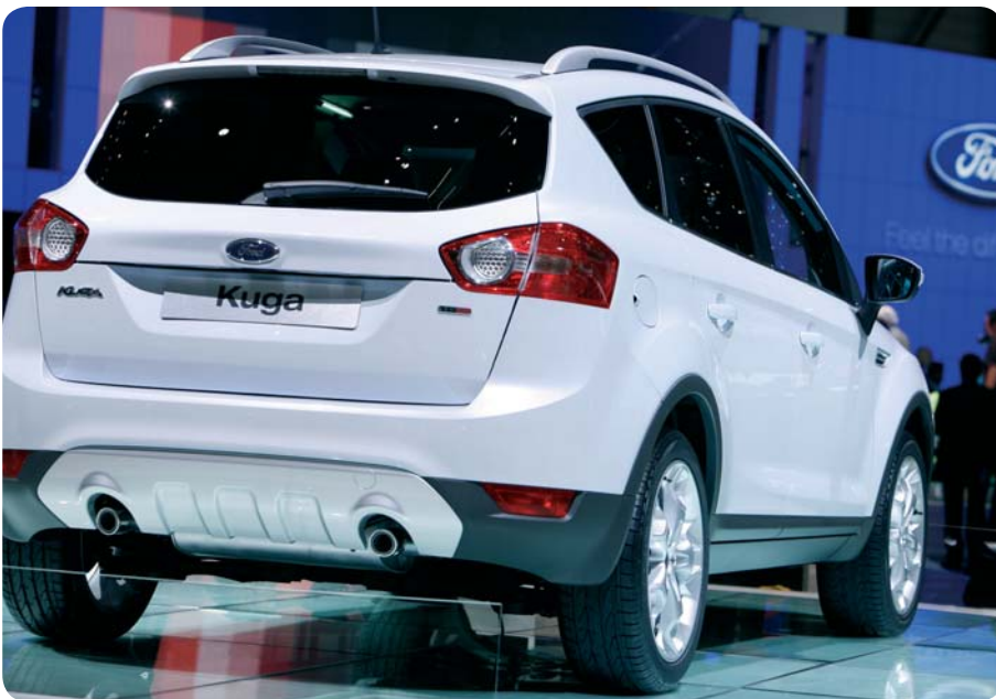
Ford Kuga roof spoiler and tailgate outer panel produced using Hifax TRC 280X
