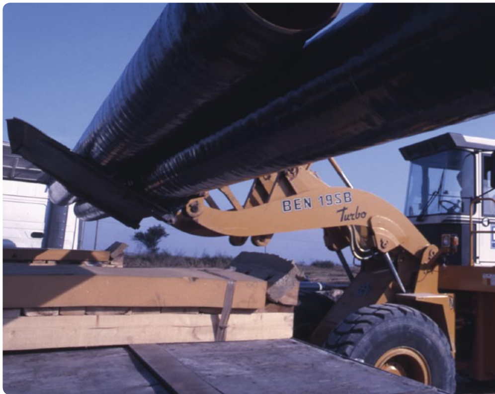
Excellent adhesion provided by Lucalen G3710E, used by customers in 3LPE coatings for gas pipelines
