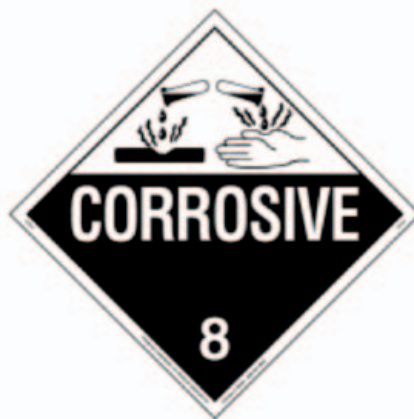
Figure 11-2 Sample of a Corrosive Material Placard
