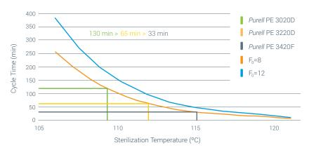
\*Ph. Eur. 5.1.5: Application of the FO concept on steam sterilization of aequeous preparations \*\*USP 24, NF19, p. 2144: Steam sterilization: "Apart from the description of the sterilization cycle, using a temperature of 121°C, the FO concept may be appropriate."
