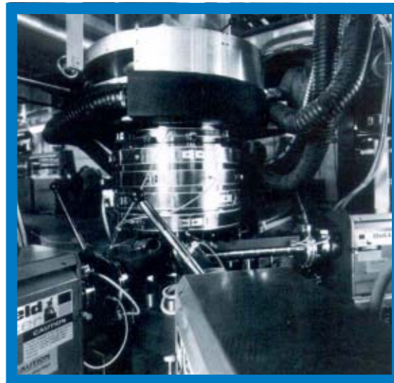
Figure 31. The compact design in this blown film system allows four coextruders to be packed into a tight space, shortening the travel distance of the melt.
