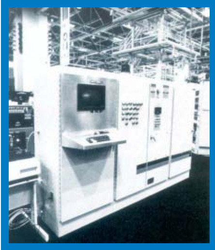
Figure 44. Microprocessor controls handle many film processing variables simultaneously.
