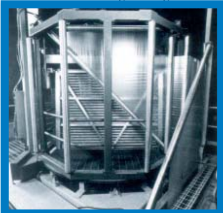
Figure 39. Oscillating (360° or 720°) haul-off units further minimize film gauge variations in the final roll.
