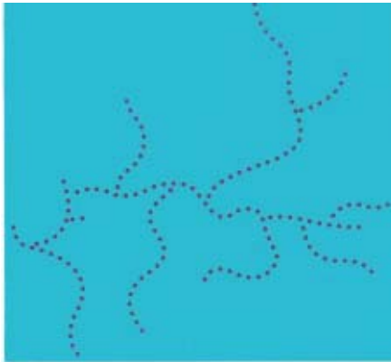
Figure 3. Polyethylene chain with side branches.
