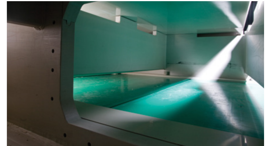
Fig. 18 - Storage tank for pickling of aluminum sheets (UHMW-PE and PP-H100) courtesy of Steuler
