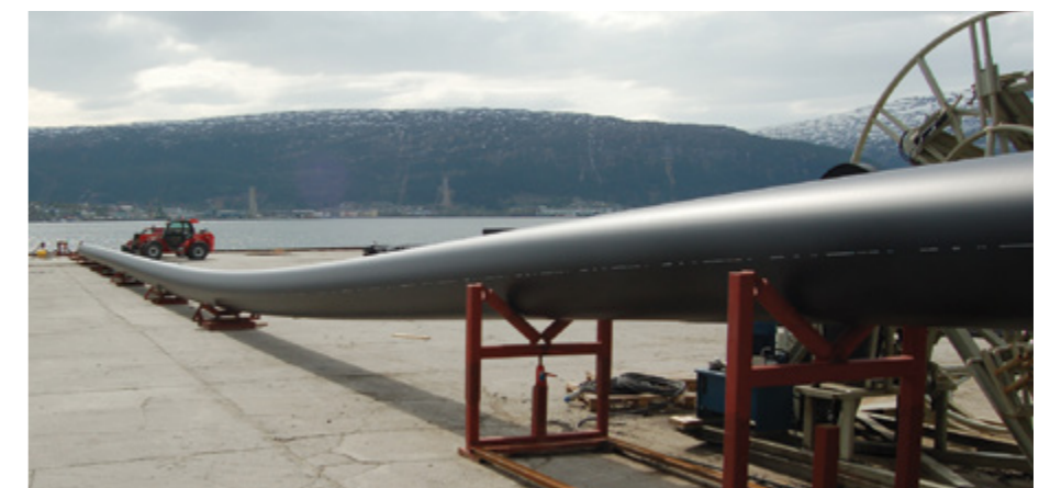
Fig. 6 - Extrusion of an 800 mm pipe
