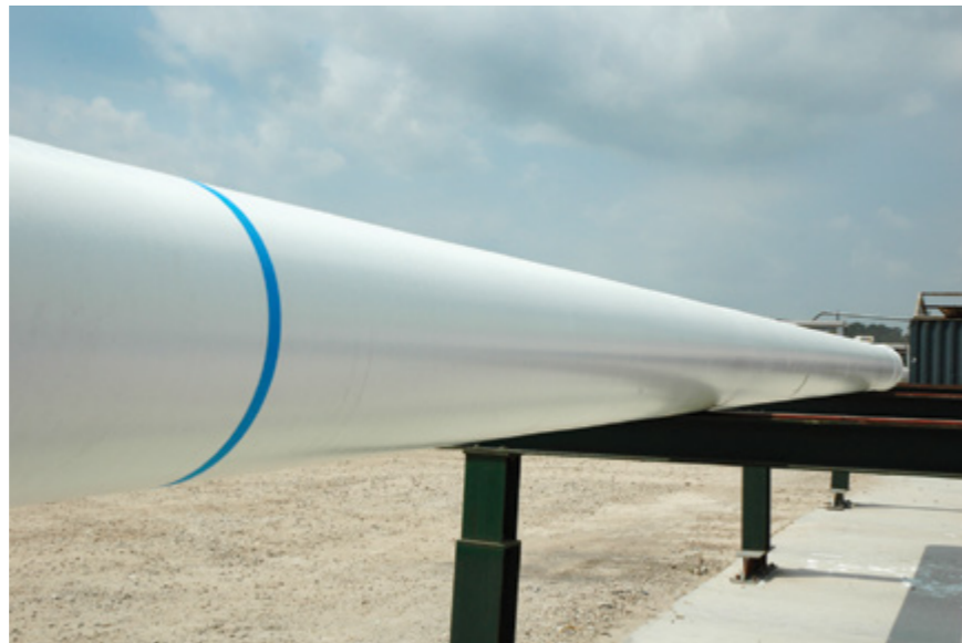
Fig. 3 - Steel pipe with PP top-coat
