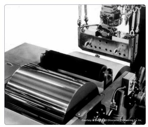
Figure 33: Cast film die and chill roll unit
