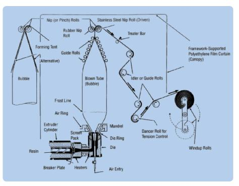
Figure 38: The blown film bubble rising up from the die is pulled into a complex takeoff system designed to yield a roll of film of high quality and uniformity.
