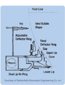
Figure 35: Dual-lip air rings blow air against the base of the bubble as well as slightly higher up.
