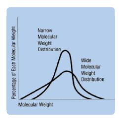
Figure 6: Schematic representation of molecular weight distribution.
