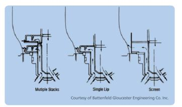
Figure 36: Internal bubble cooling (IBC) systems direct the air flow onto the inside surface of the bubble. There are three basic types: (1) a stacked air ring with multiple annular gaps at different levels; (2) a single-lip ring; and (3) a screentype air ring that applies a large volume or air through a large open area.
