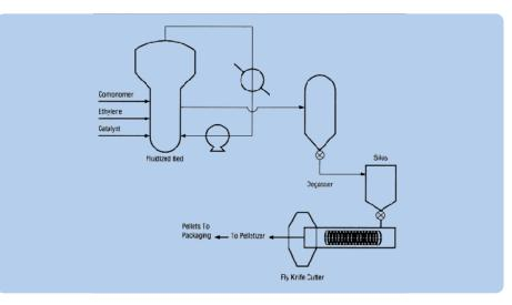
Figure 11: Process diagram for LLDPE or HDPE production in a gas-phase reactor.
