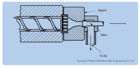
Figure 24: Schematic of a pressure valve.
