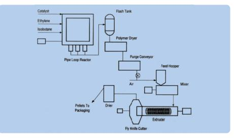
Figure 10: Process diagram for HDPE production in a particle-form reactor.
