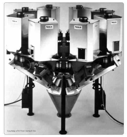
Figure 17: Gravimetric feeder/blender with eight ingredient modules.
