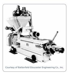
Figure 15: The extruder consists of a resin feeding hopper, a heated barrel, a constant rotating screw, a manual screen changer, a die adapter and a base.
