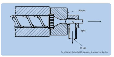
Figure 26: Film extrusion involves the melt passing through transfer piping. The length of this piping must be as short as possible.
