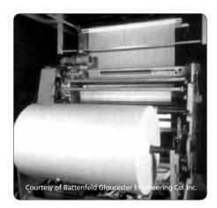
Figure 41: Surface winders have a rotating drum that forces the film roll to turn and, thus, wind up the film web.
