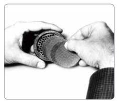
Figure 21: Breaker plate (left) and screen pack.
