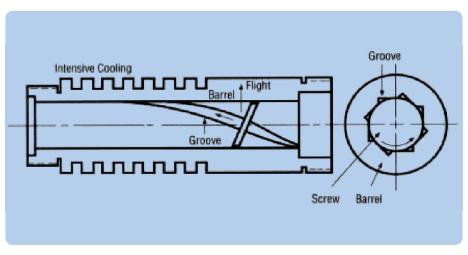
Figure 18: For HMW-HDPE and LLDPE film extrusion, barrels are designed with up to 12 helical grooves.
