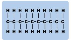
Figure 2: Polyethylene molecular chain.
