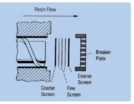
Figure 22: Schematic of a screen pack and breaker plate assembly.
