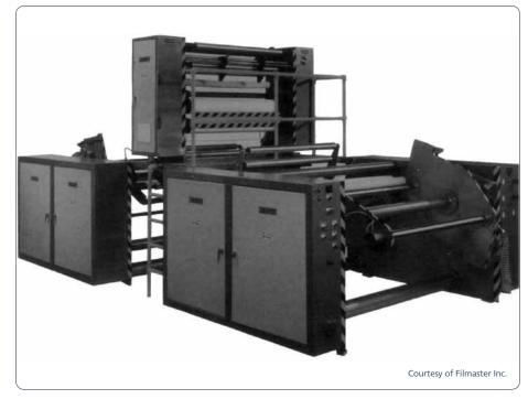
Figure 42: Turet winders are designed to rotate a full film roll out of contact with the lay-on roll and index a new core into the winding position.
