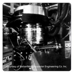
Figure 31: The compact design in this blown film system allows four coextruders to be packed into a tight space, shortening the travel distance of the melt.
