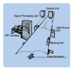
Figure 40: Optical inspection systems, located above the frost line of the bubble, check for film imperfections during extrusion.
