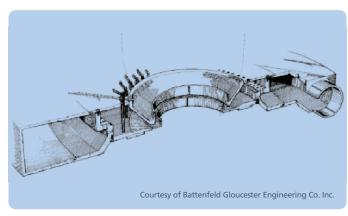
Figure 34: An air ring around the exiting polyolefin tube just above the die is the most common means of solidifying and cooling the bubble.
