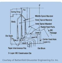
Figure 30: Schematic of a blown film coextrusion die design with multiple mandrels.
