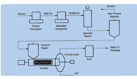
Figure 9: Process diagaram for LDPE production in an autoclave reactor.
