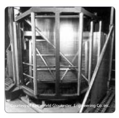
Figure 39: Oscillating (360° or 720°) haul-off units further minimize film gauge variations in the final roll.
