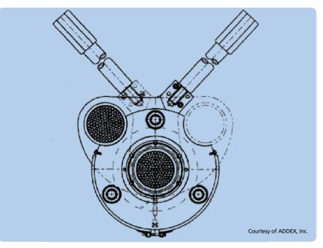
Figure 23: A manual screen changer is the most commonly found type in the industry.
