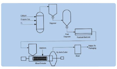
Figure 12: Process diagram for PP production in a vertical, stirred fluidized bed, gas-phase reactor.
