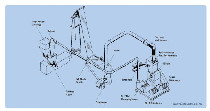
Figure 43: Edge trim, start-up waste, trim made during slitting, etc. can be recycled in-line, an important capability for source reduction programs.
