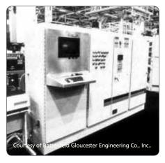
Figure 44: Microprocessor controls handle many film processing variables simultaneously.
