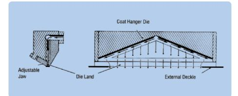
Figure 32: Schematic cross section on a "coat hanger"- type cast film die.
