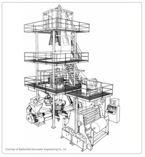
Figure 16: Coextrusion systems designed for making multilayer film have two or more extruders feeding a common die assembly.
