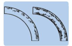
Figure 13: Interior surfaces of long radius blends should be roughened to minimize "angel hair" and streamer formation in transfer systems.
