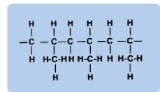
Figure 3: Polyethylene chain with side branches.
