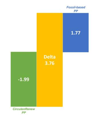
The use of *Circulen*Renew PP reduces the CO<sub>2</sub>eq emissions by **3.76 tons CO<sub>2</sub>eq per ton** of PP vs equivalent fossil fuel based polypropylene
