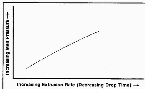
**Fig. 1: Melt Flow as Expected**
