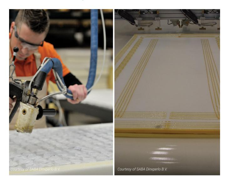
The assembly of spring-loaded mattresses requires an excellent green strength\* combined with a long open time to allow a manual or automated assembly process.
