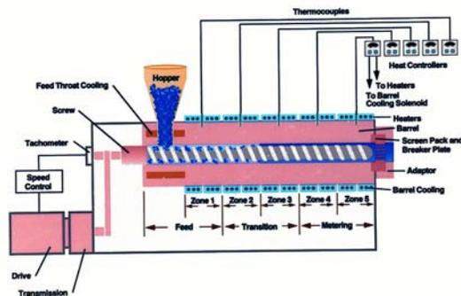
In some cases a screen pack and breaker plate are positioned at the end of the barrel to filter out foreign contaminants that may have entered the hopper. The screen pack also increases backpressure in the barrel,
