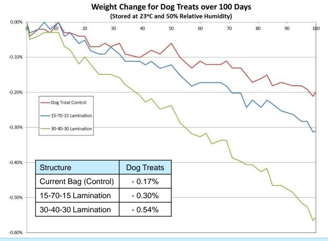
Higher HDPE content leads to structures that approach the weight change of the control bag and may be sufficient for some applications
