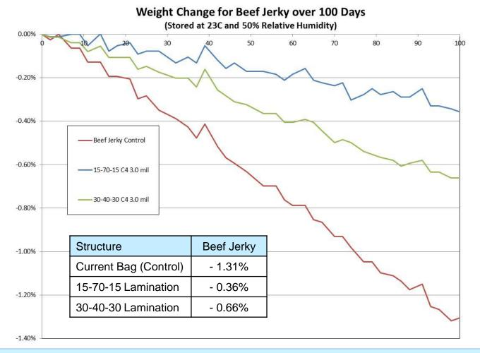
Barrier lamination structures appear to show significantly less weight change over time than current package
