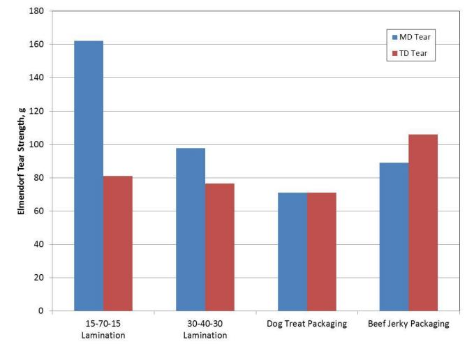
**Barrier Lamination structures have comparable tear**
