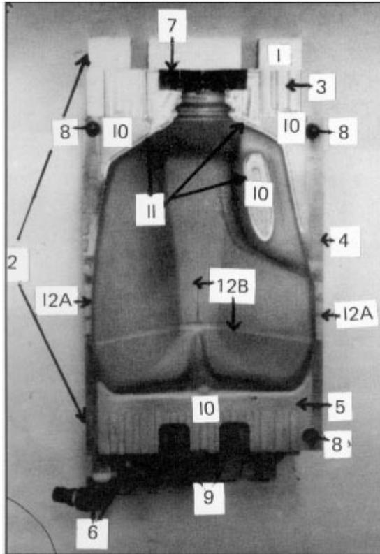
1. Backing plates that allow for easy mounting of cavities to movable platens. These platens incorporate slots in the top and bottom for slight adjustments vertically and horizontally.
