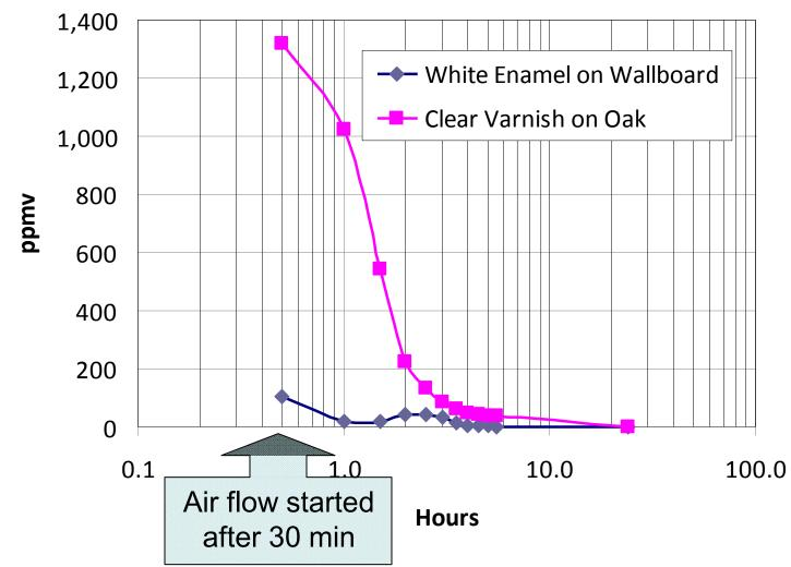
Samples placed in chamber immediately after roller application of two coats.
