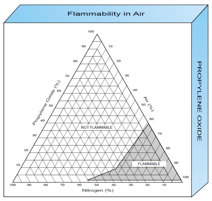
To determine if a mixture of propylene oxide is flammable, find the concentration of propylene oxide and the air or nitrogen concentration. Follow both lines until they intersect. If they intersect within the shaded area, the mixture is flammable.
