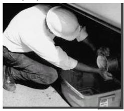
Figure 11. Hopper car delivery: inspecting the unloading tube and placing a filter and catch pan.
