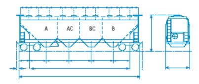
Figure 2. A typical hopper car is divided into four compartments.
