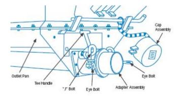
Figure 13. Basic components of an adjustable pneumatic outlet.
