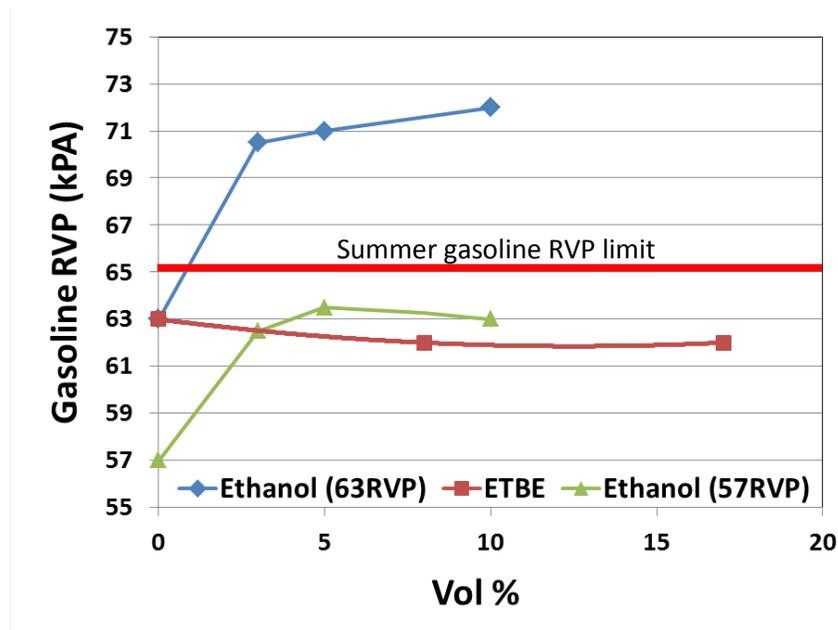
**Figure 3:** Effect of Ethanol and ETBE on the RVP of Blendstocks for Oxygenated Blending (BOB). Ethanol BOB RVP must be reduced by 6-10 kPa for finished gasoline to meet summer specification. In contrast, the same base gasoline can be used with ETBE.
