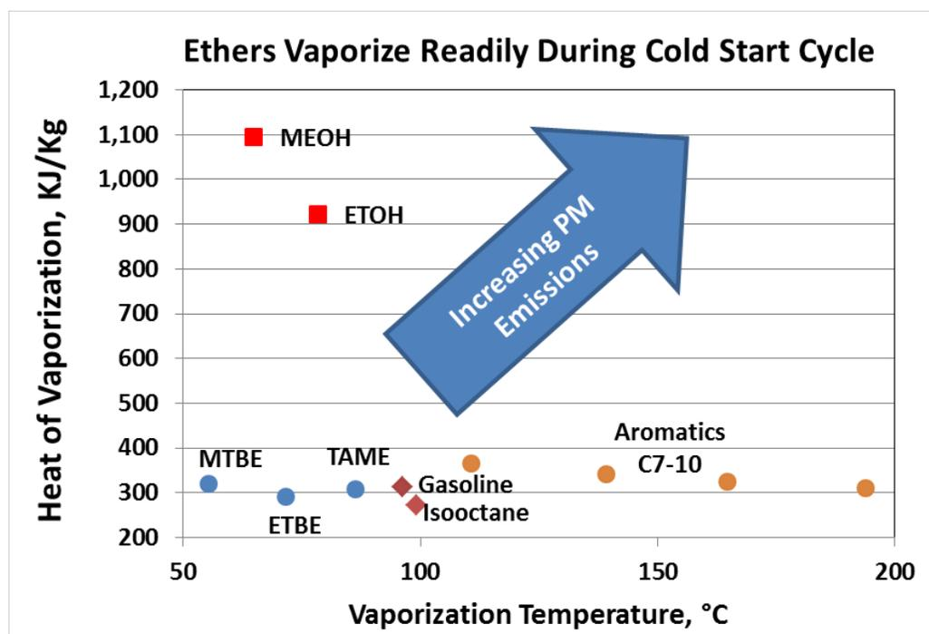
**Figure 7:** Heat of Vaporization vs. Boiling Point of Common Gasoline Blending Components. Aromatics do not completely vaporize under cold-start conditions, increasing hydrocarbon and particulate emissions and reducing fuel efficiency.
