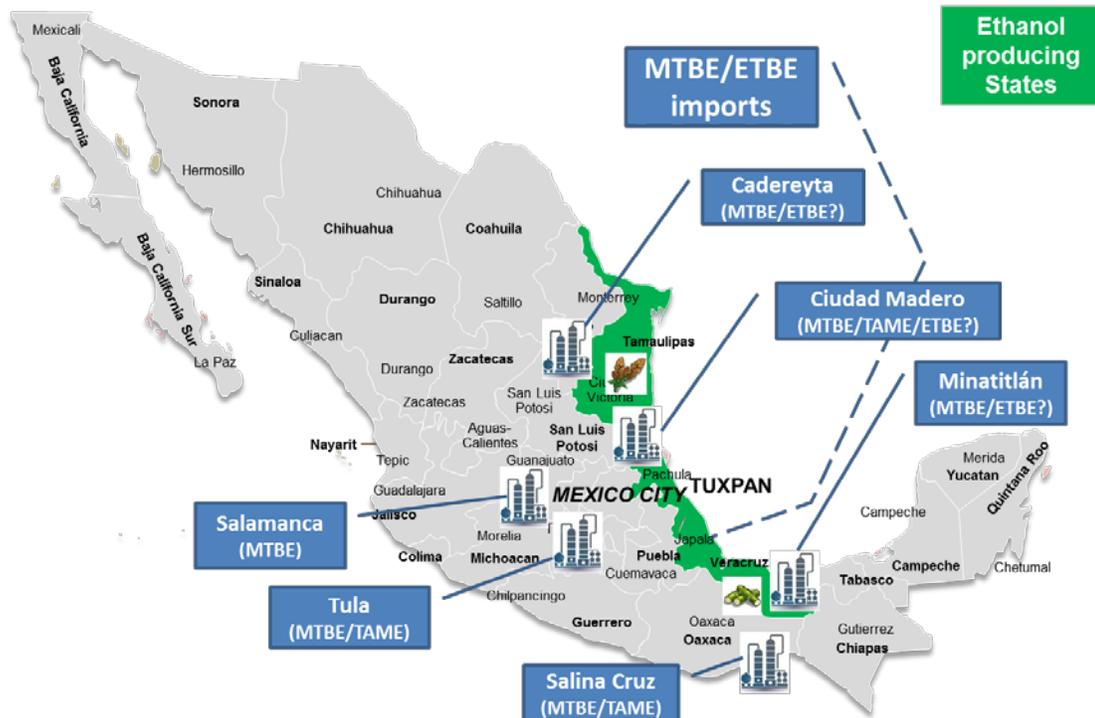
**Figure 10:** Domestic Ethanol from Veracruz and Tamaulipas could be converted to ETBE at local refineries with minimal capital investment compared to converting the current gasoline distribution system to handle ethanol blending at terminals and running refineries at higher severity.
