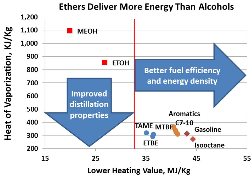
**Figure 8:** Heat of Vaporization vs. Lower Heating Value of Common Gasoline Blending Components. Alcohols require more heat to vaporize and contain less energy than ethers and other gasoline components. This reduces fuel efficiency and increases tailpipe emissions.
