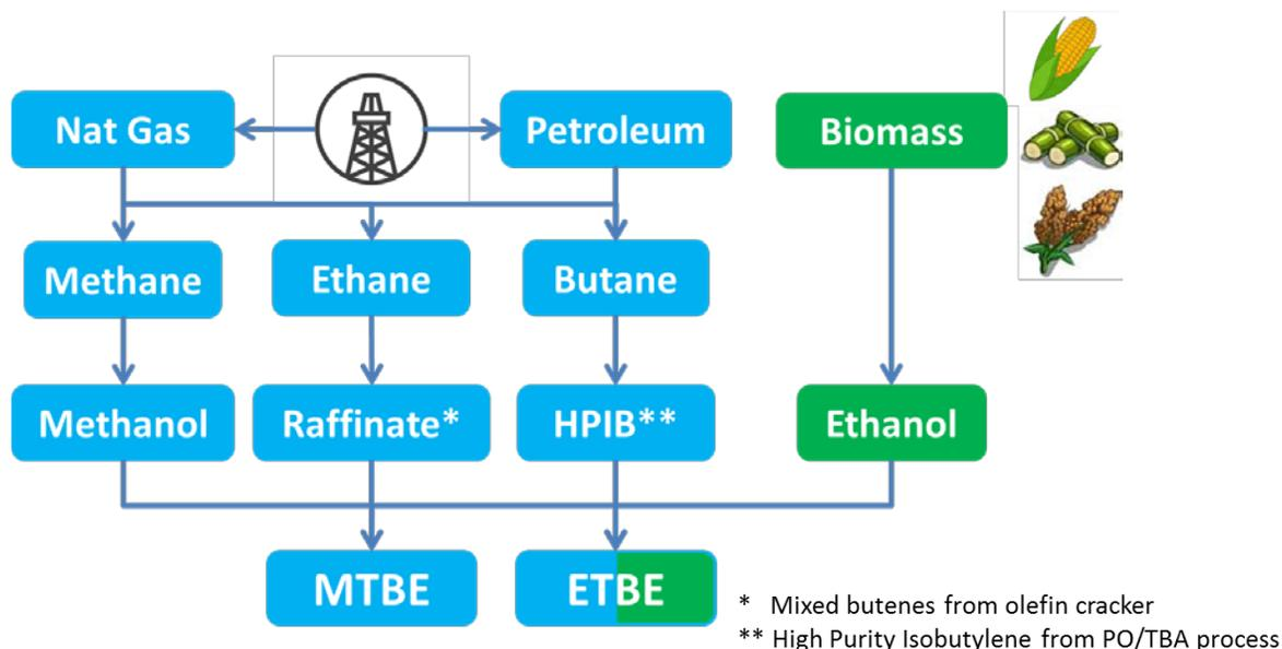
**Figure 11:** Raw materials and intermediates in the production of MTBE and ETBE. Main crops for bioethanol include corn, sugarcane, and sorghum.
