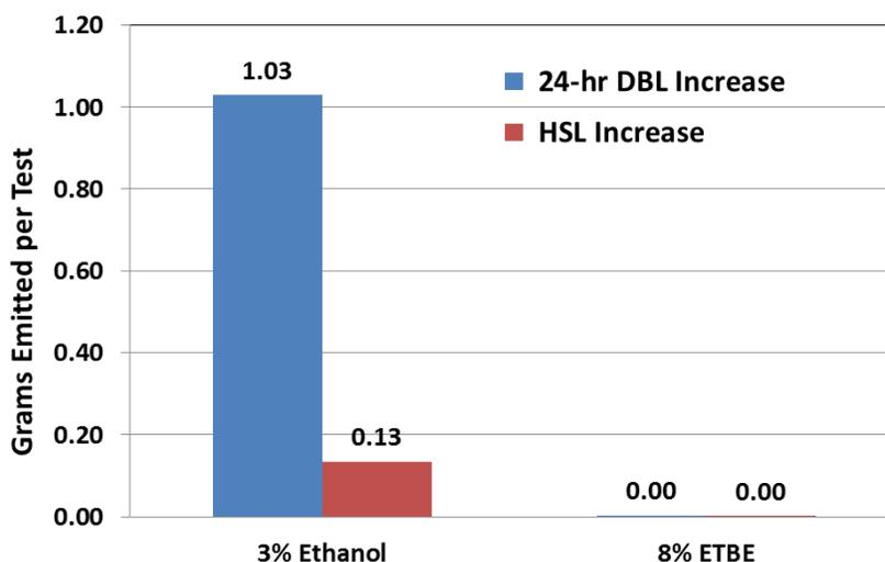
**Figure 4:** Effect of 3% Ethanol and 8% ETBE on Fugitive Emissions from Vehicle Fuel Systems.
