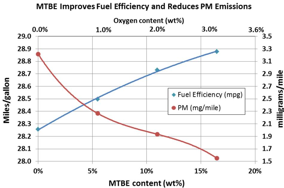
Figure 9: Effect of increasing MTBE Content on PM Emissions and Fuel Efficiency in a Modern Gasoline Direct Injection (GDI) Engine under NDEC and FTP-75 Protocols.
