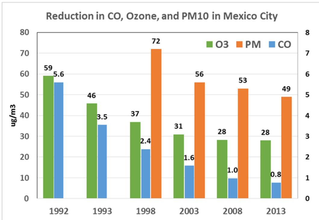
Figure 1: Reduction in the Air Pollutants Carbon Monoxide (CO), Ozone, and Particulate Matter (PM10) in the Valley of Mexico following the adoption by PEMEX of MTBE as an oxygenated gasoline component in 1992. Red Automática de Monitoreo Atmosférico (RAMA) database.
