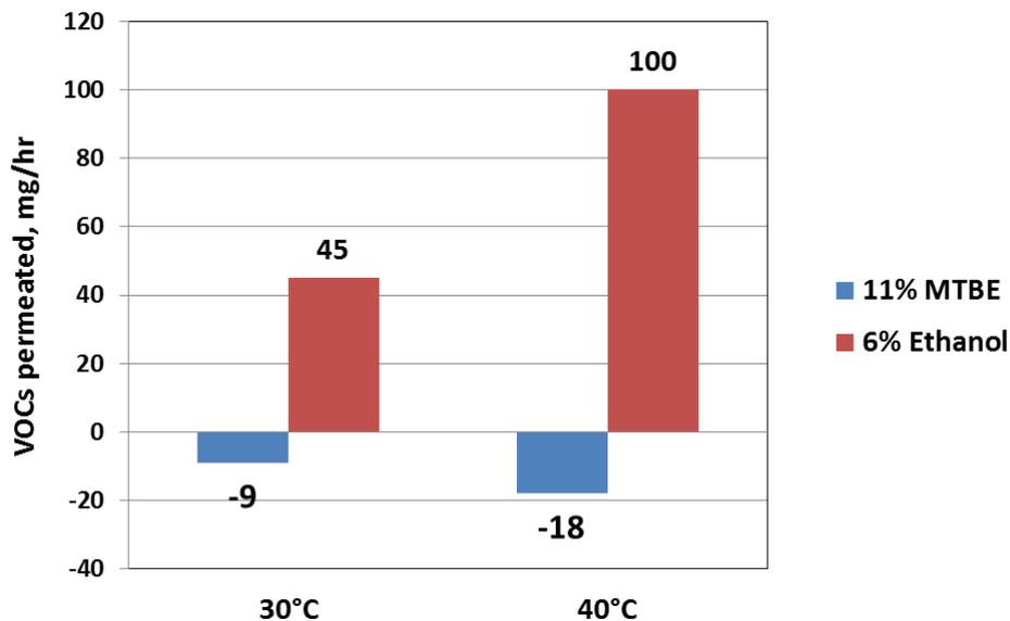
**Figure 5:** Average (10 vehicles) effect of adding 5.5% ethanol and 11% MTBE on static fugitive VOC emissions from gasoline compared to similar gasoline without oxygenates.
