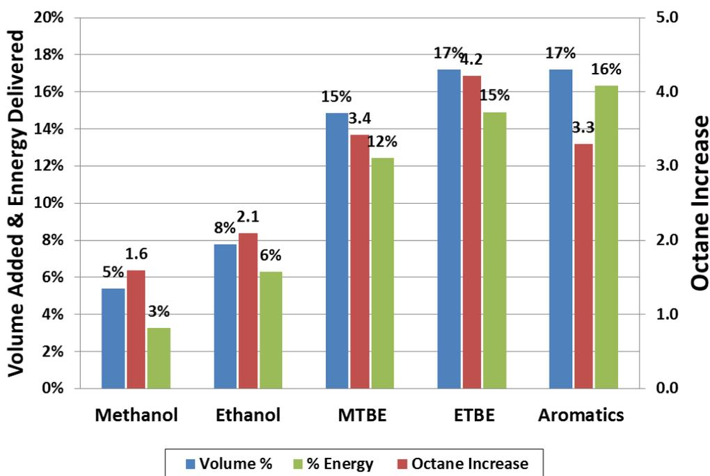
**Figure 13:** Comparison of the octane, volume, and energy contribution of alcohols vs. ethers at the same oxygen content (2.7 wt. %) and aromatics on the same volume basis as ETBE (17 wt. %).
