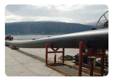
Alathon L5008HP is a bimodal, high molecular weight, high density polyethylene resin with excellent processing characteristics. With a melt index of 0.07 g/10 minutes, Alathon L5008HP will process as easily as a product with a higher melt index of 0.1 g/10 minutes. As a result, higher machine throughput or lower horsepower and head pressure can be achieved by using this resin.
