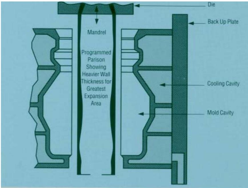
**Figure 27. A programmed parison designed to fit a particular mold configuration.**
