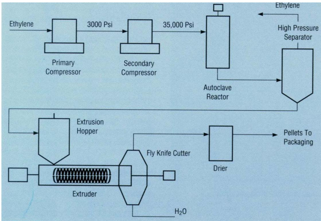
Figure 10. Process diagram for LDPE production in an autoclave reactor.
