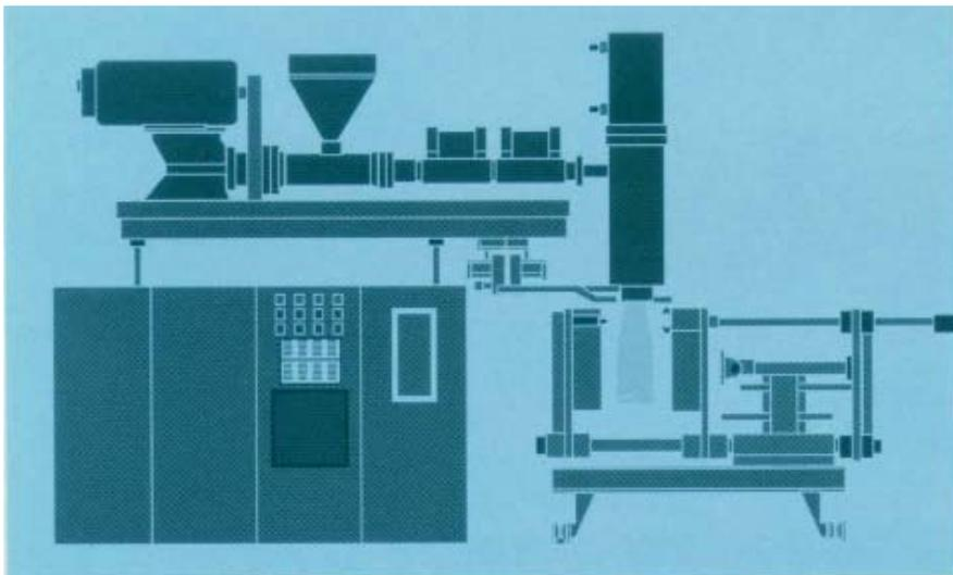
**Figure 37. Continuous extrusion, accumulator head.**
