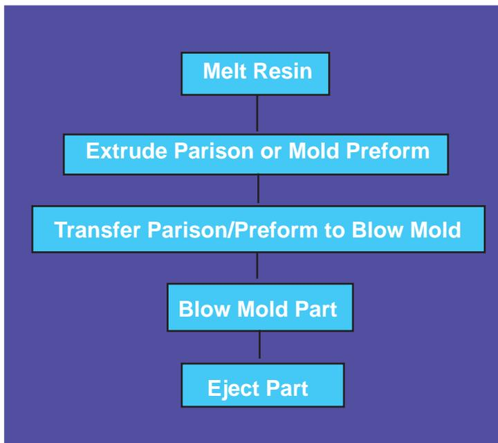
**Figure 16. The five steps in the blow molding process.**
