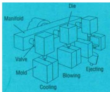
Figure 25. Multiple-dies, multiple-stationary-mold equipment.
