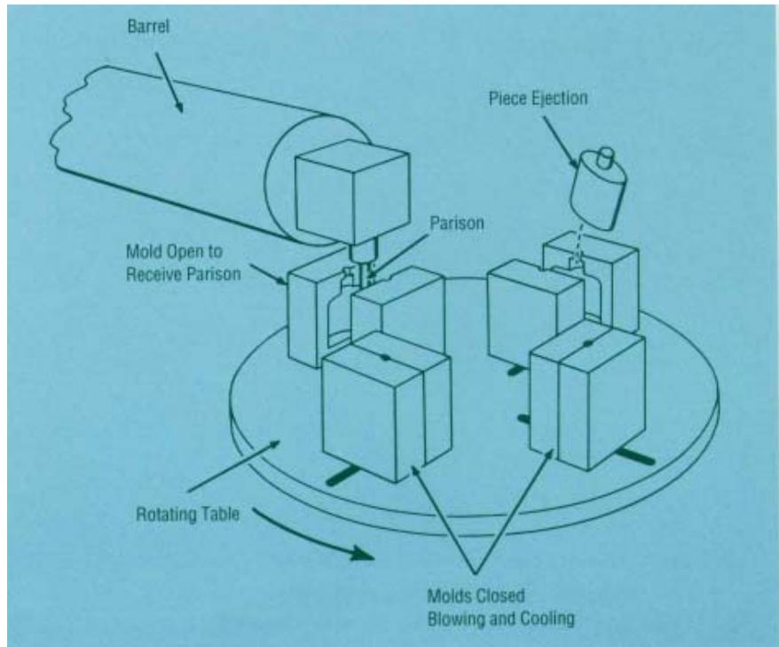
Figure 32. Multiple-station turntable.
