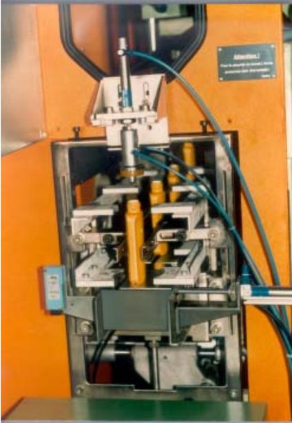
**Figure 50. Testing bottles for leaks using an air pressure system.**
