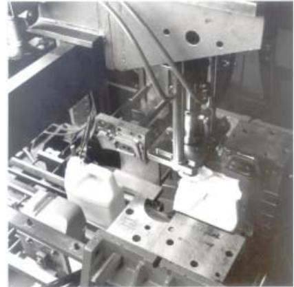
**Figure 48. Containers are finished in the machine and oriented to stand-up position for take-away conveyers.**
