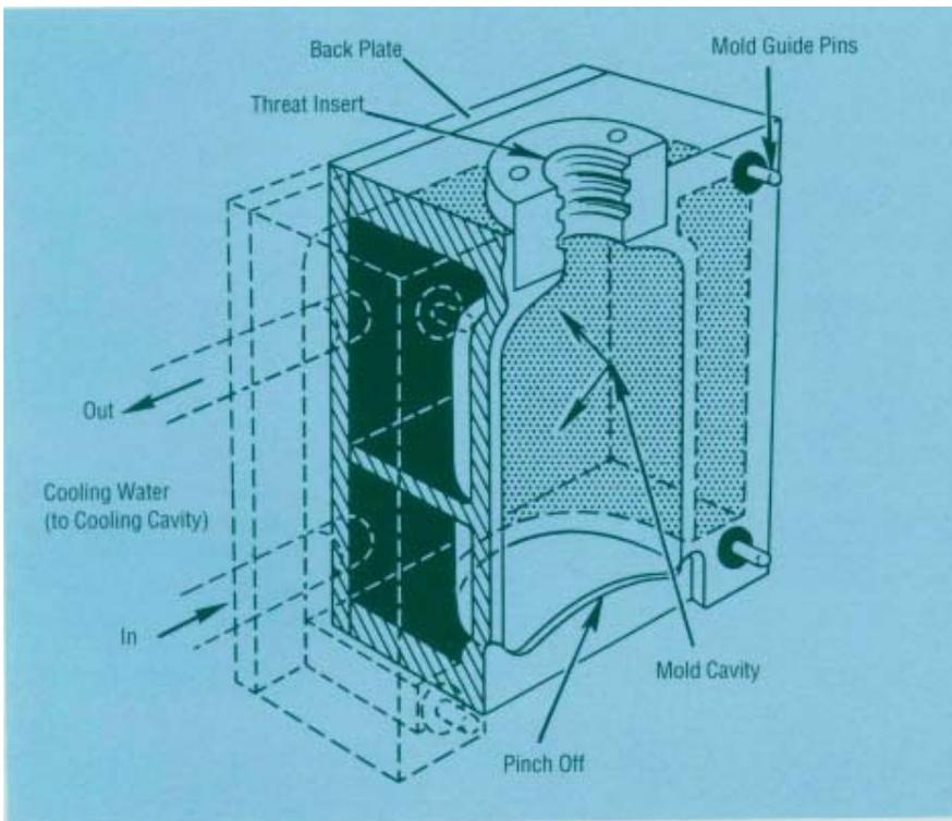
Figure 47. Schematic of a blowing mold half, with the cooling water channels indicated.
