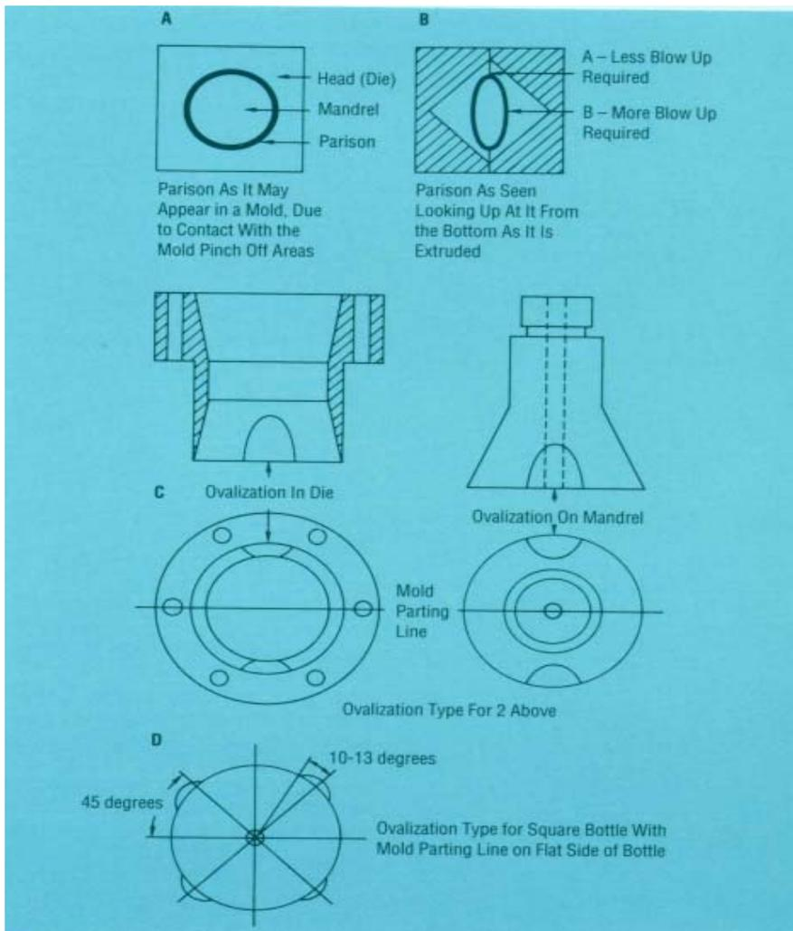
Figure 57 A schematic representation of ovalized tooling.
