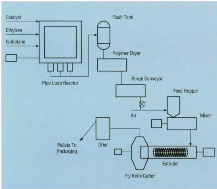
Figure 11. Process diagram for HDPE production in a particle-form reactor.
