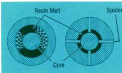
Figure 23. Left: perforated (breaker plate); Right: spider (cross-piece type of core support in a blow molding die).
