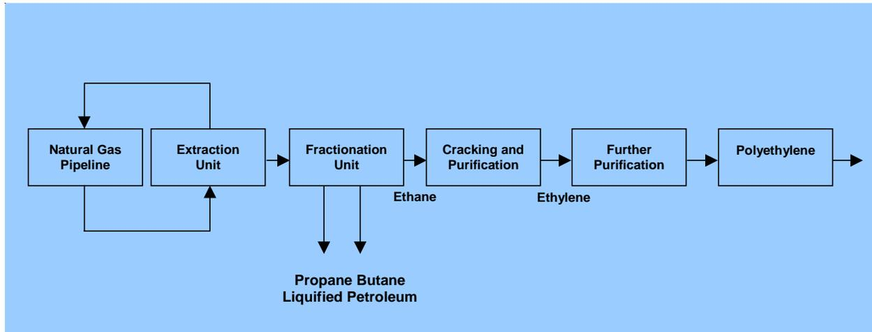
Figure 8. Diagram of the polyethylene process from natural gas to resin pellets.
