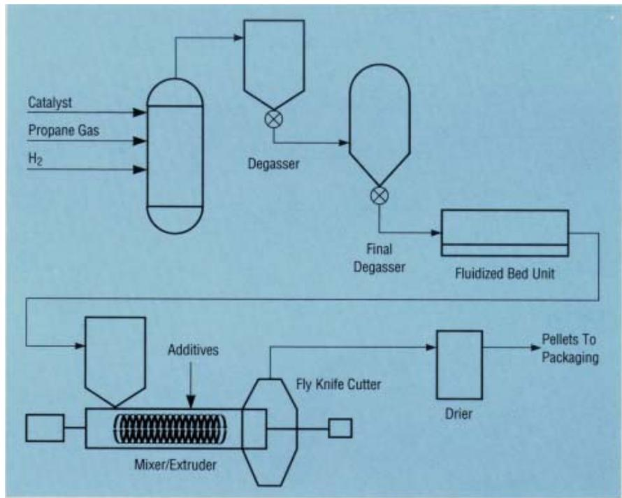
Figure 13. Process for polypropylene production.
