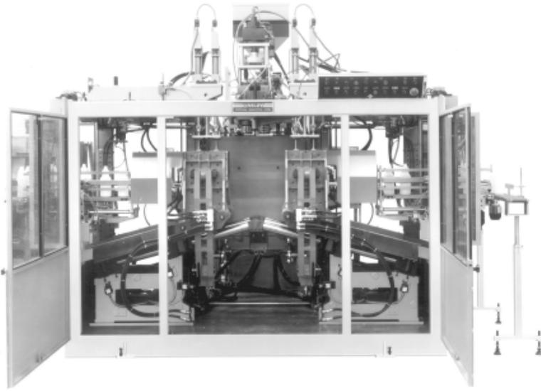
**Figure 34. Continuous extrusion blow molding machine with a shuttle mold carrier.**
