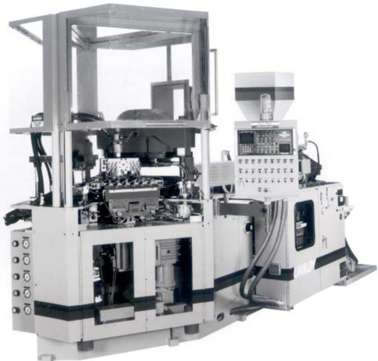
**Figure 60. Injection blow molding machine**
