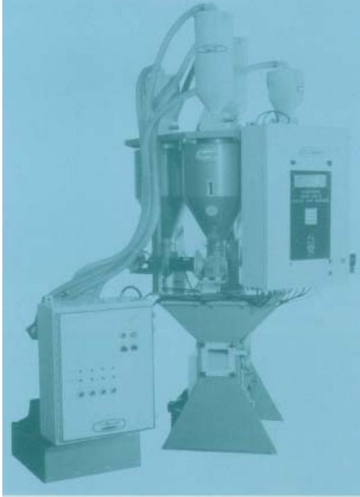
**Figure 15. Gravimetric blending units accurately measure components in polyolefin extrusion.**
