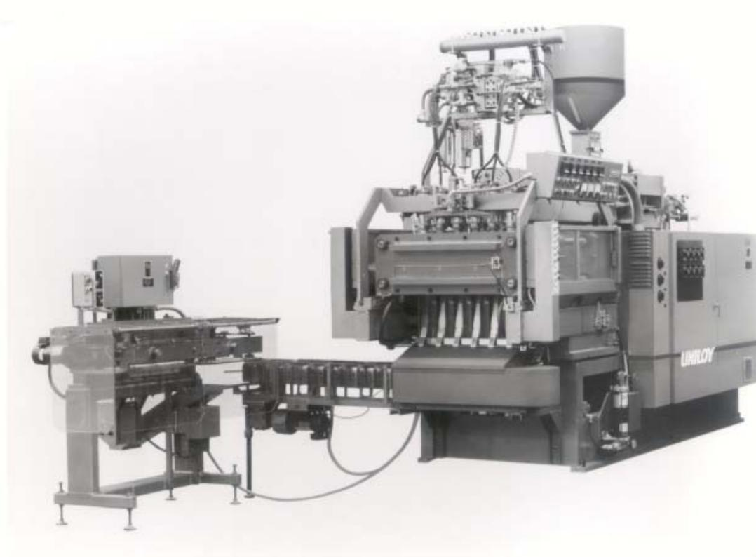
**Figure 40. Reciprocating screw extrusion blow molding system.**
