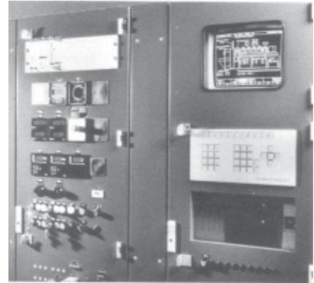
**Figure 28. Control unit for a parison programmer.**
