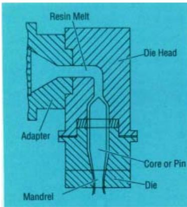
Figure 22. Schematic of center-fed die.
