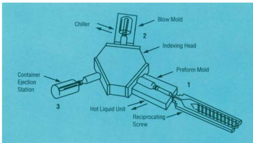
Figure 58. Injection blow molding.
