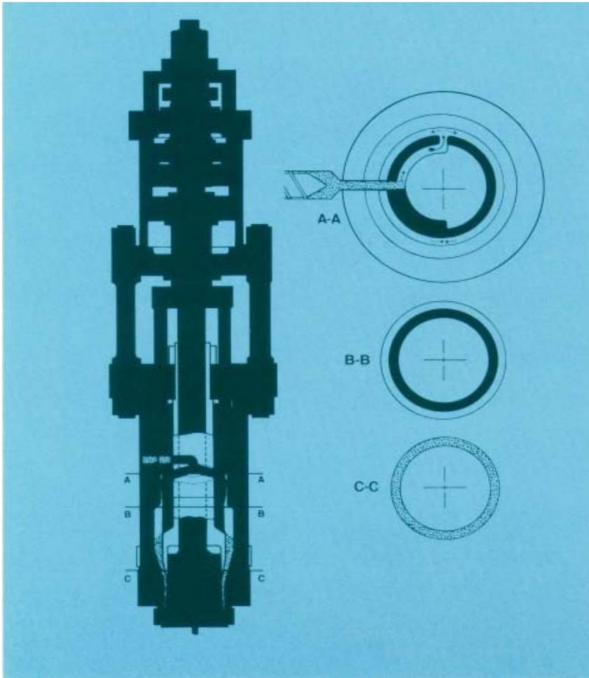
Figure 38. Example of an accumulator used for blow molding large parts.
