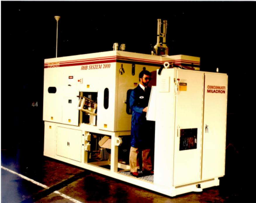
**Figure 61. Two-stage injection blow molding machine.**
