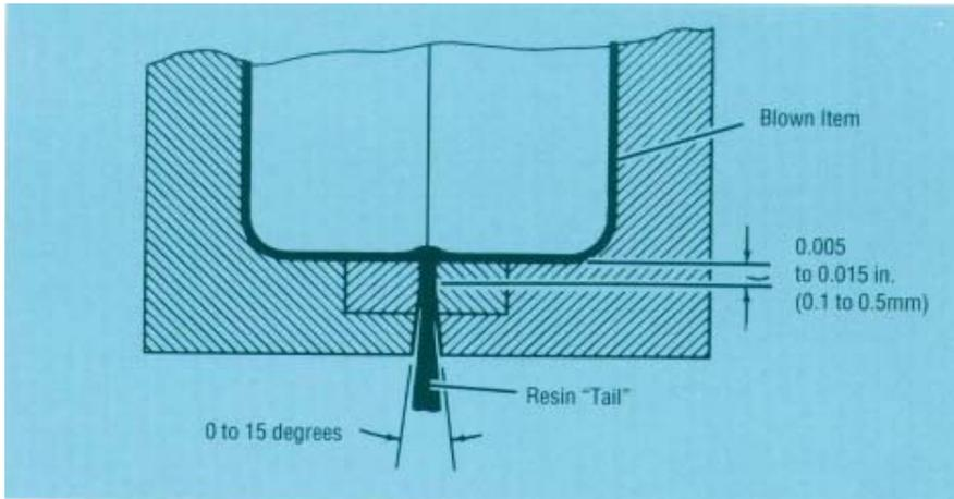
Figure 44. Shape of a pinch-off with insert as recommended by some molders.
