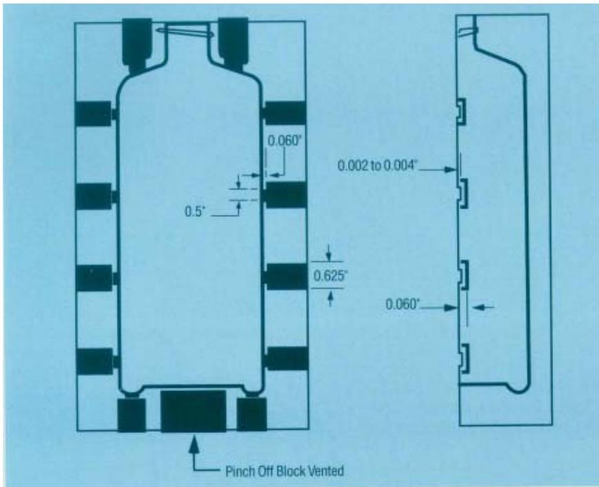
Figure 46. Mold Venting
