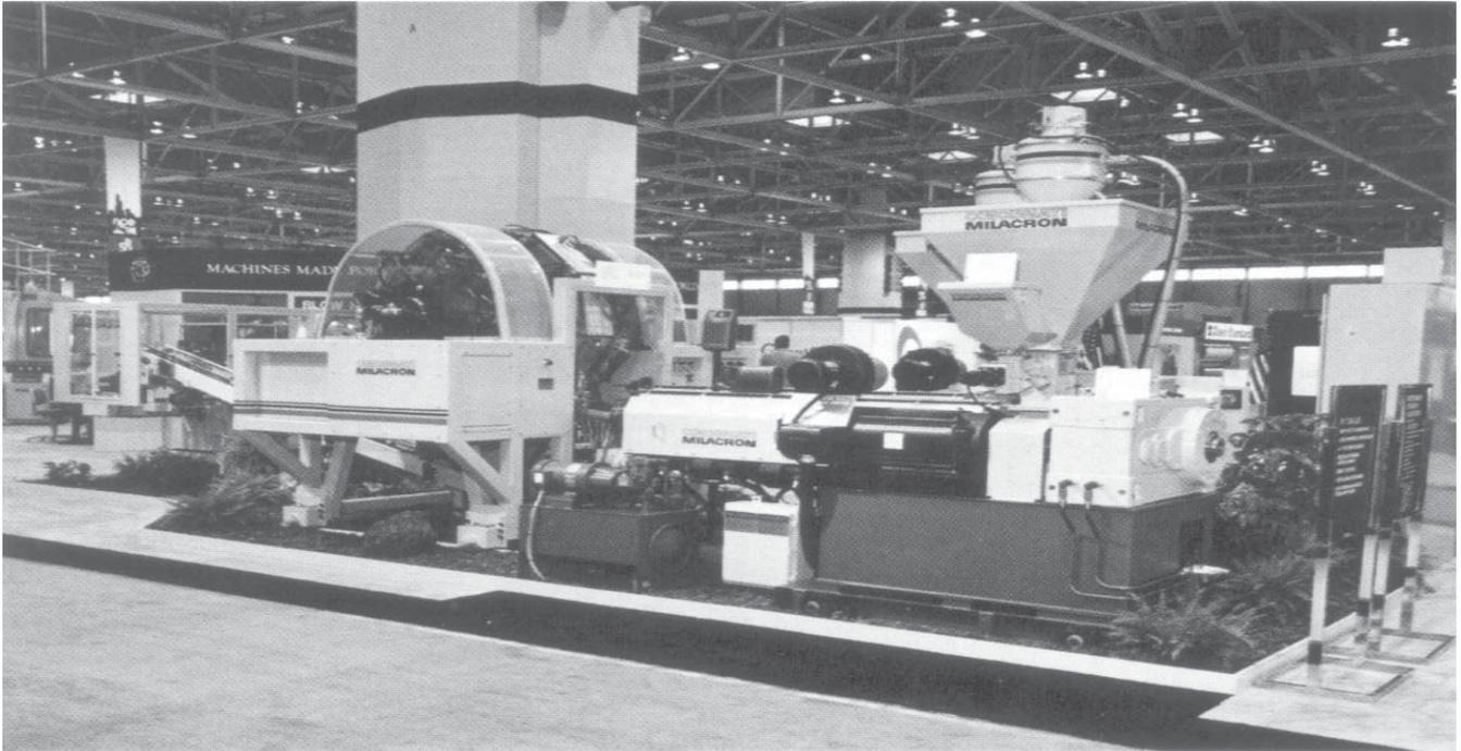
Figure 30. A rotary blow molding machine
