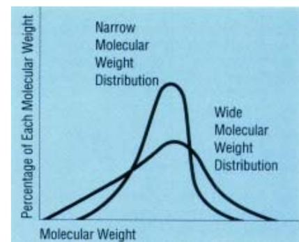
**Figure 7. Schematic representation of molecular weight distribution.**
