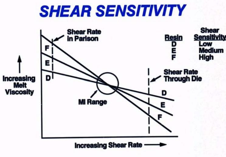
**Figure 6.** The importance of good shear sensitivity—high viscosity in the parison, low viscosity through the die.
