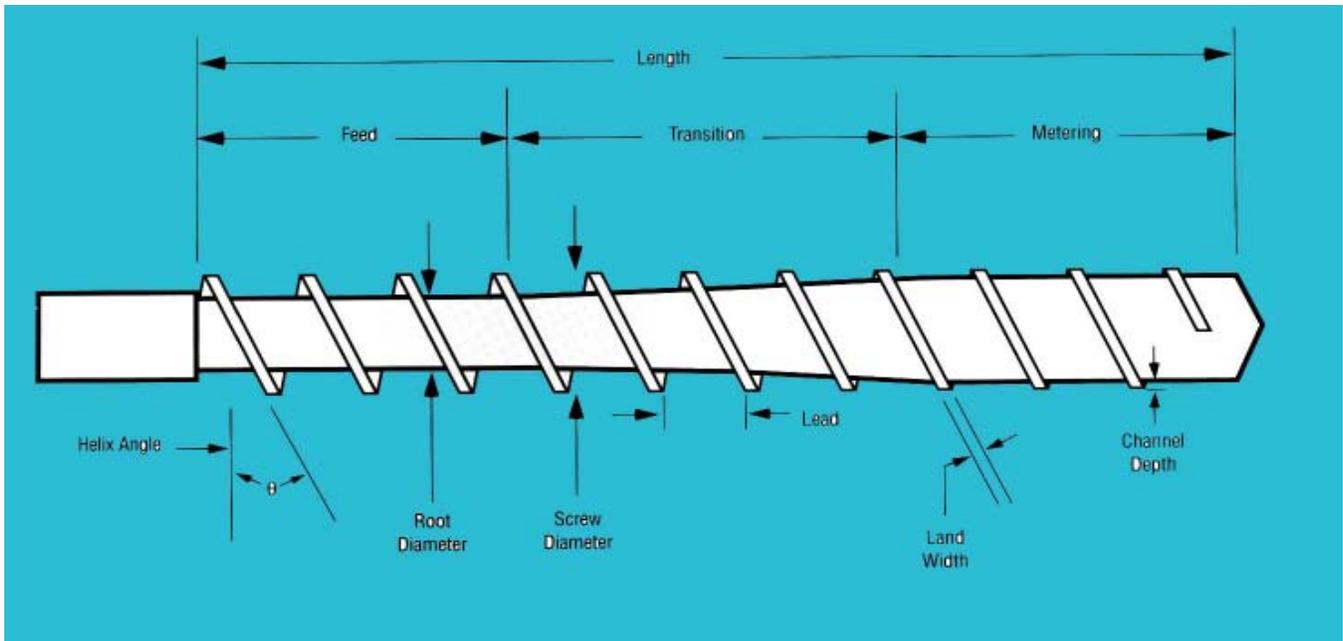
Figure 19. Typical extruder screw for HDPE
