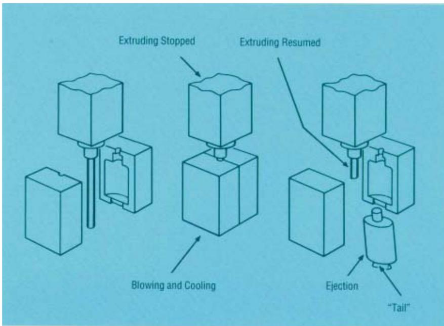
**Figure 36. Schematic of intermittent parison extrusion into a stationary mold. Extruder operation is interrupted after the parison has reached the desired length and before the mold halves have closed around it (left). Operation is resumed only at the end of the ejection step (right).**
