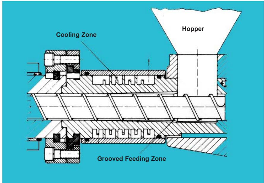
Figure 18. A cross section of the extruder barrel.
