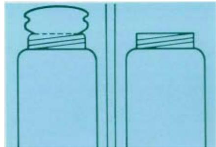
**Figure 49. A knife trimmer cuts the “dome” off wide-mouthed, blow molded containers.**
