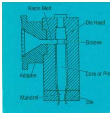
Figure 24. Schematic drawing of a side-fed die with a grooved core.
