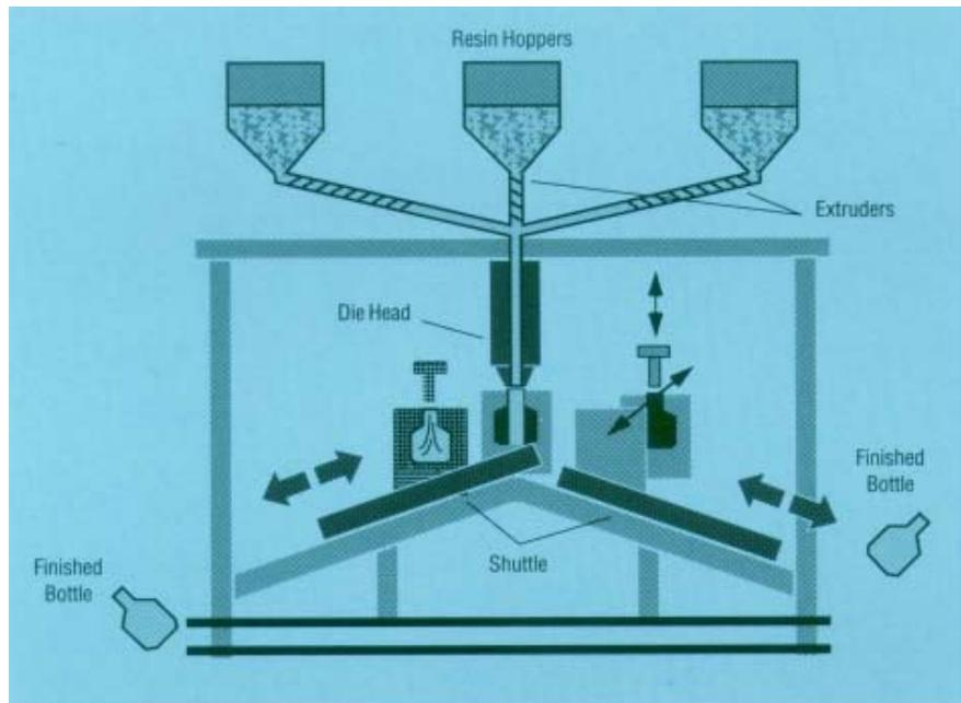
Figure 33. Continuous extrusion blow molding machine, with a shuttle system.
