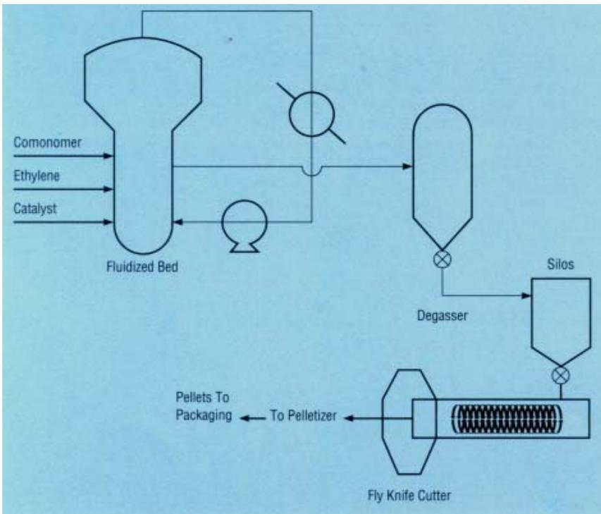
Figure 12. Process diagram for LLDPE production in a gas-phase reactor.
