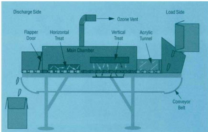
Figure 53. Electronic corona-discharge treatment.
