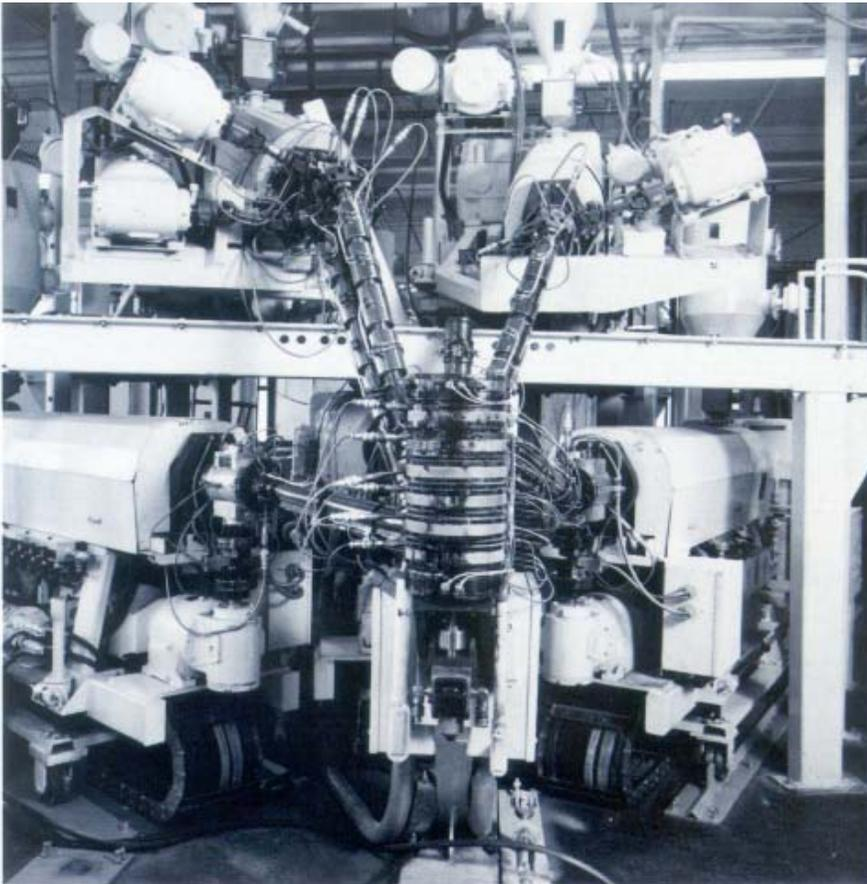
**Figure 29. Multiple extruders and special die heads are needed for coextruded multiple-layer bottles.**
