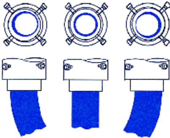
Figure 56: Adjusting die bolts to prevent parison curving.
