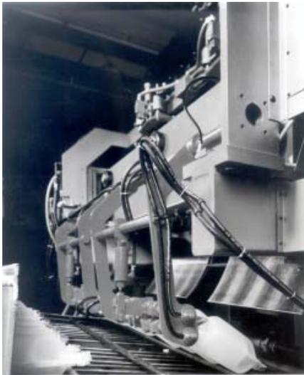
**Figure 51. Take off equipment on a blow molding machine**
