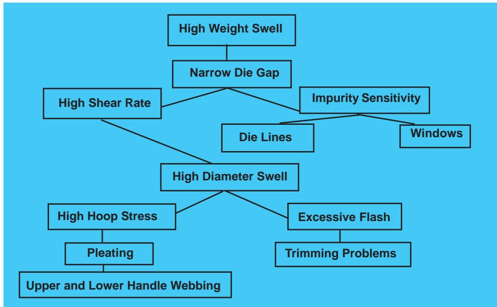
Figure 55. Problems encountered in counteracting high weight swell.
