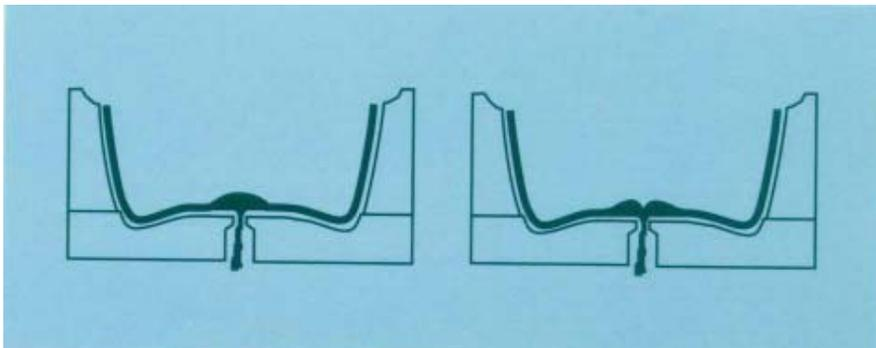
Figure 45. Good weld (left) and poor weld (right).
