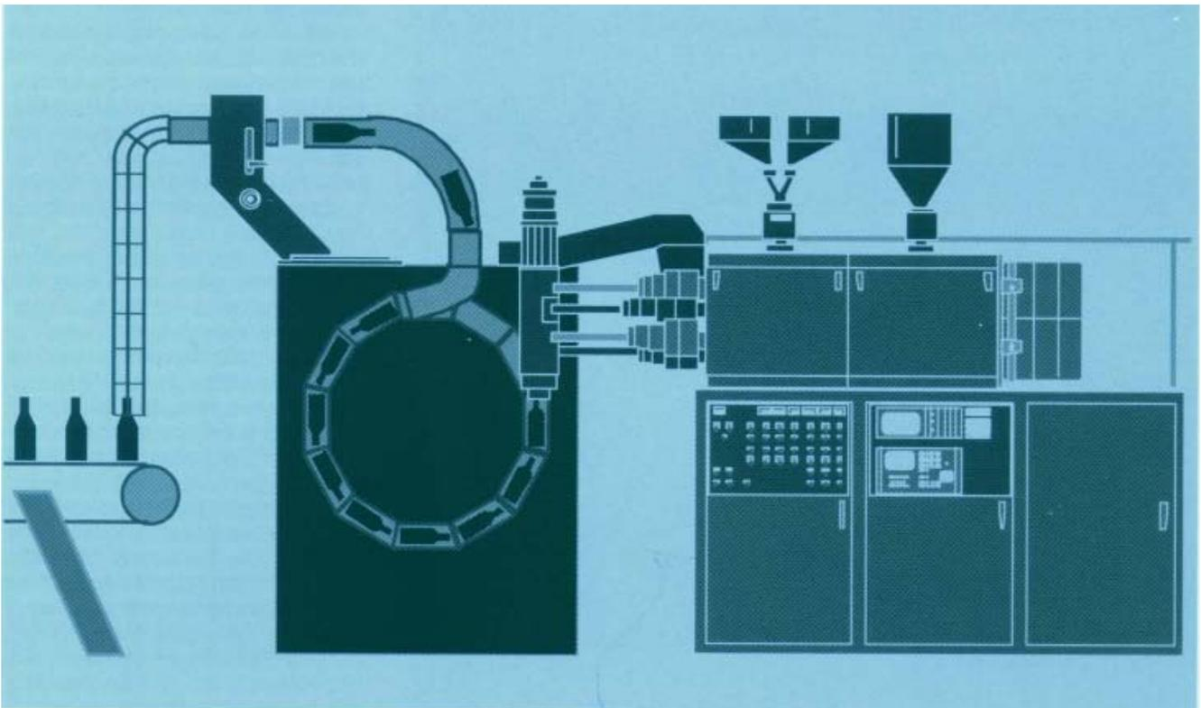
Figure 31. Continuous extrusion blow molding machine with a vertical wheel.
