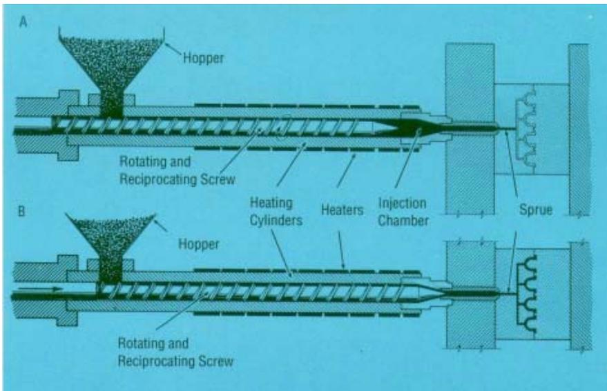
Figure 39. Schematic cross section of a typical screw injection molding unit showing the screw in the retracted (A) and the forward (B) position.
