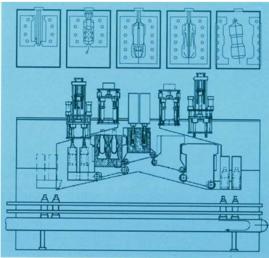
**Figure 35. Extrusion stretch blow molding.**
