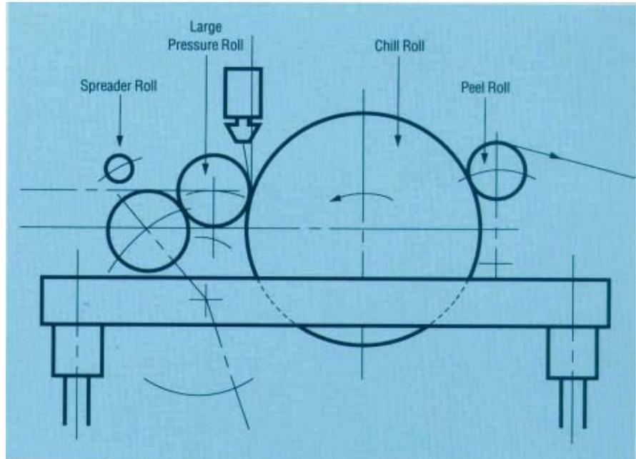
Figure 40. Coating Station (set air gap range for 5” minimum to 15” maximum)
