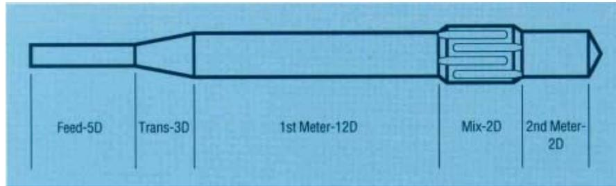
Figure 26. Mixing Screw
