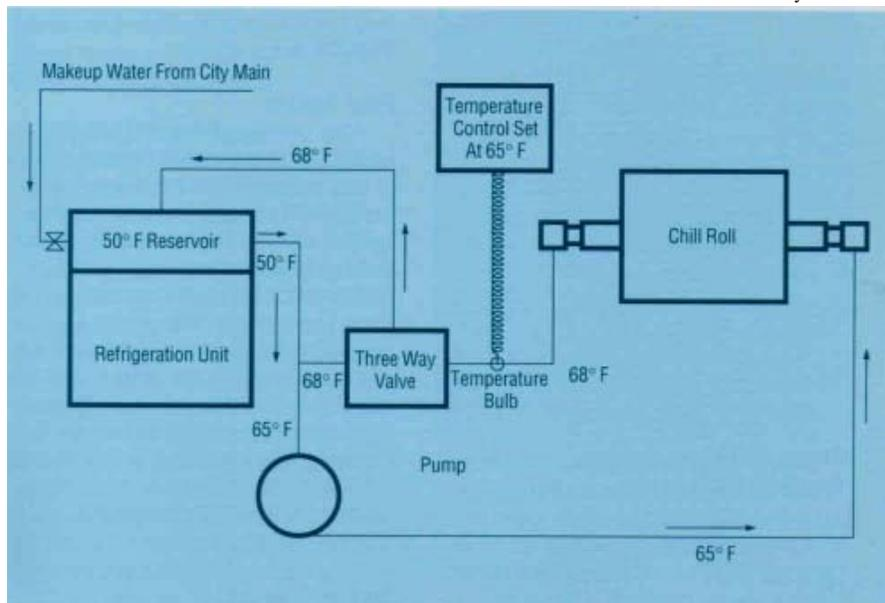
**Figure 42. Closed Circuit Chill Roll Cooking System**
