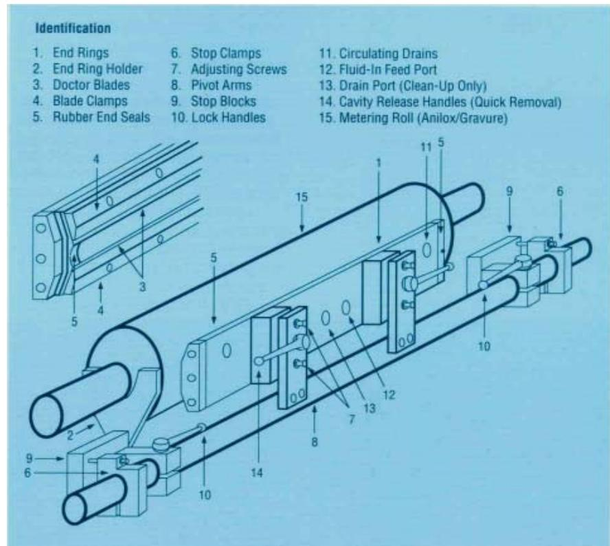
Figure 20. Reverse Angle Dual Blade Applicators for Priming
