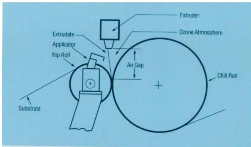
**Figure 18. Ozone air is generated in a remotely located ozone chamber and carried through flexible hose to the applicator which distributes the ozone air evenly over the entire width of the extrudate.**
