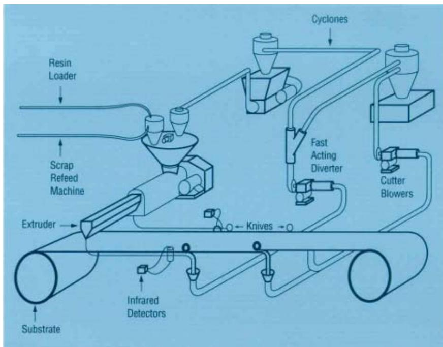
Figure 48. Extrusion Coating Scrap Recycle System
