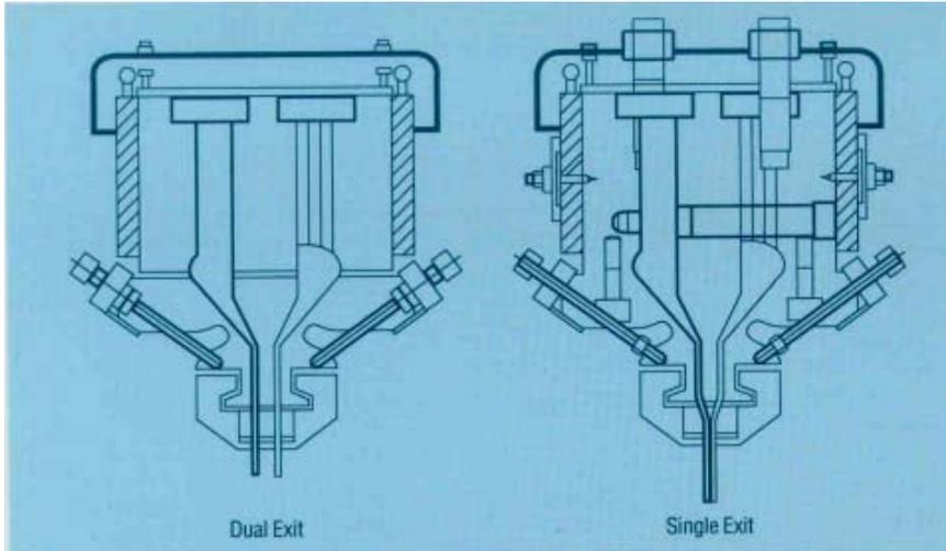
Figure 37. Designs of Manifold Dies
