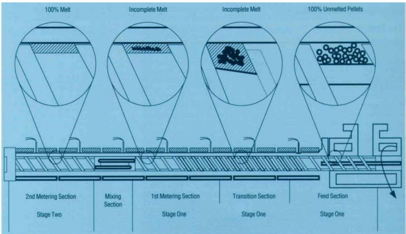
Figure 25. Extruder Cross Section with Polymer Melting Stages
