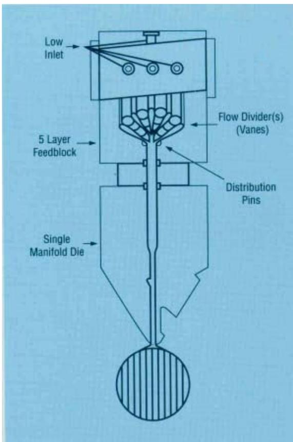
Figure 38. Coextrusion Coating Feedblock and Monolayer Die
