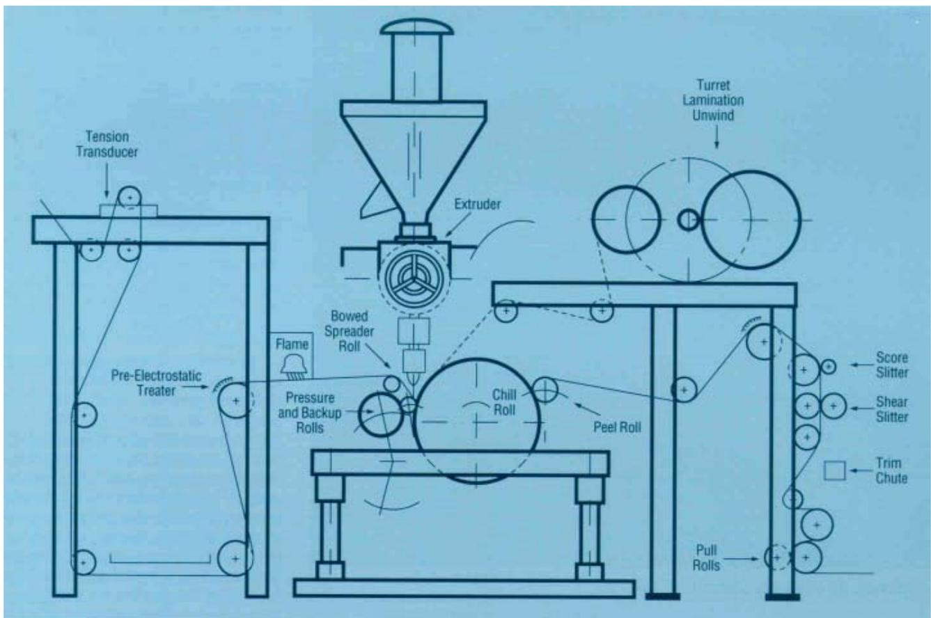
Figure 41. Extrusion Lamination Machine and Trim Slitting Station
