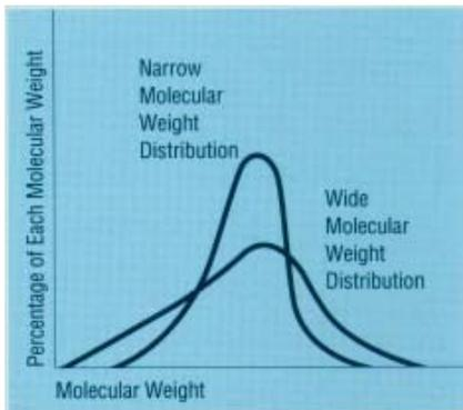
**Figure 5. Schematic representation of molecular weight distribution.**
