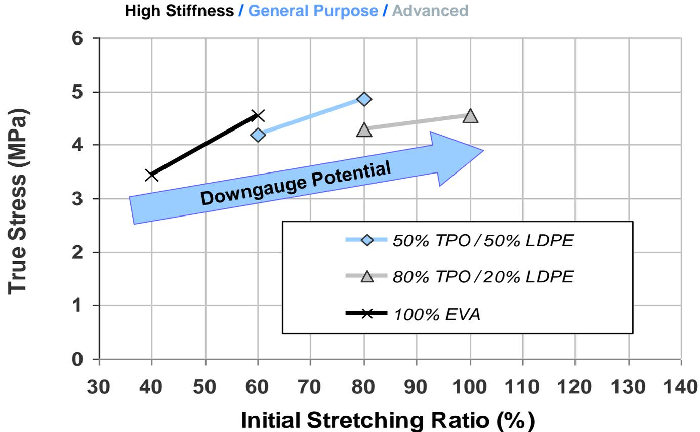
\*Residual Stress' divided by 'Film Thickness on load' times 'Initial film thickness' (80µm)
