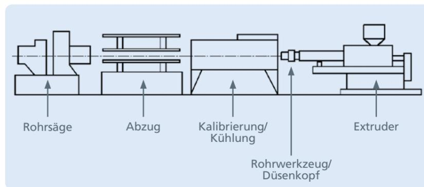
Fig. 2: Production process for extruded pipes as per DIN 8074
