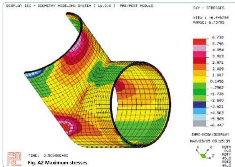
Fig. 7: Finite element model, tee DN 1400, LGA Nuremberg <sup>6</sup>
