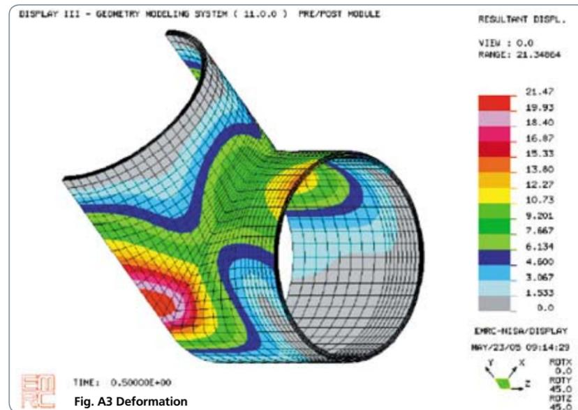
Fig. 8: Finite element model, tee DN 1400, LGA Nuremberg <sup>6</sup>
