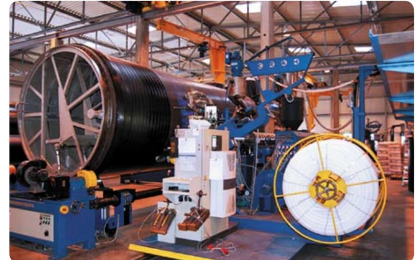
Fig. 3: Production of spirally wound pipes at FRANK & KraH GmbH as per PAS 1065 / DIN 16961
