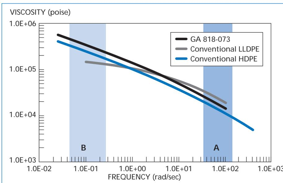
All polyethylene resins display a phenomenon known as shear thinning. As a resin is pushed faster through an extruder at high shear rates (high frequency), it appears to have a decreasing viscosity. The amount of “shear thinning” that occurs is largely controlled by the breadth of the resin’s molecular weight distribution. Broad molecular weight distribution resins display greater shear thinning, which translates into easier extrusion.
