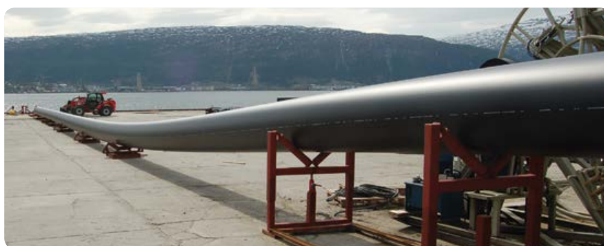
Fig. 6 – Extrusion of an 800 mm pipe
