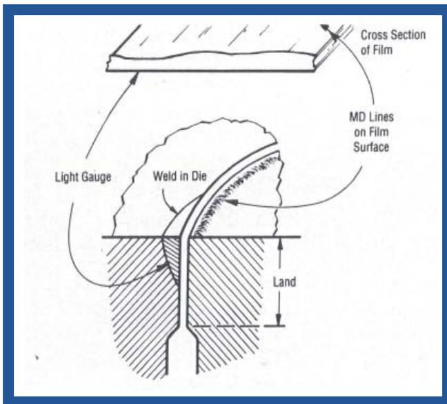
Figure 17: A gauge band results from the weld in the die lip. The build-up on the die lip drags and marks the film surface.
