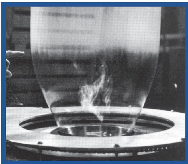
Figure 16: A well-shaped bubble with horizontal frost line visually indicates good gauge control.
