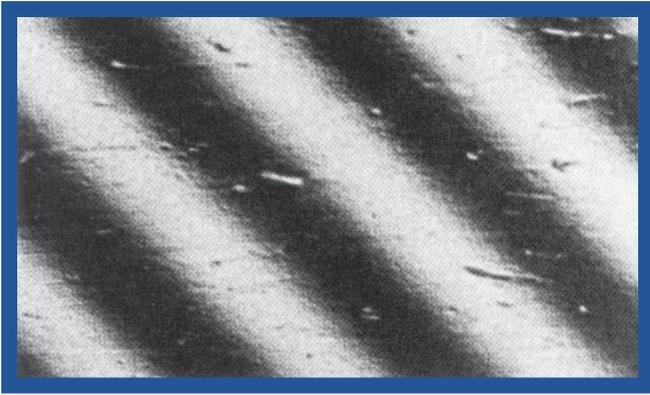
Figure 21: Gels were caused by moisture getting into resin when delivery truck was unloaded in the rain.
