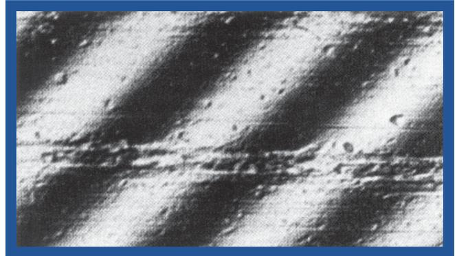
Figure 22: Severe die lines indicate that a dirty die is the probable source of gels in the film.
