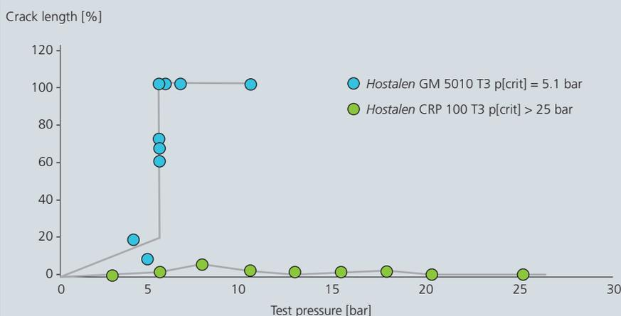
The results of the S4 test showed that pipes in *Hostalen* CRP 100 Black retain their stability up to a pressure of 25 bar; no rapid crack propagation takes place (Tests performed by: Gastec, Netherlands) [3]
