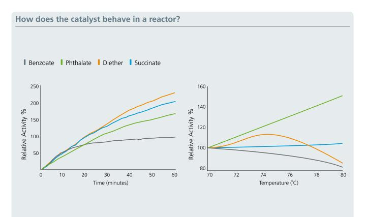
A complete understanding of catalyst kinetic behaviour is key to ensuring good plant performance
