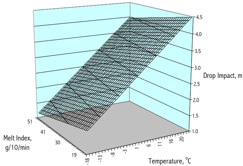
Figure 6. Drop Impact as a Function of MFR and Temperature
