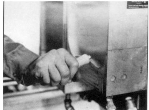
*Figure 2: Apply the tool with both force and judgment to sharpen worn pinch-offs.*
