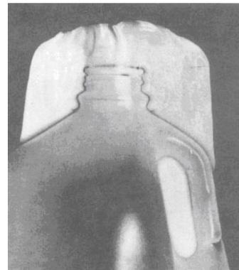
**Figure 4: With the flash ending far too high on the handle, a blowout and a useless bottle result.**
