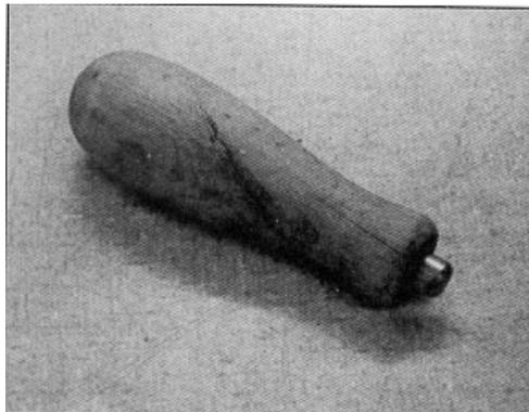
*Figure 1: An improvised, pinch-off, reworking tool made from a drill rod and a discarded file handle.*
