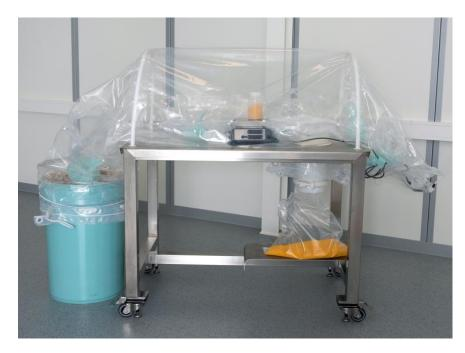
Material Transfer System for contained bag charging & discharging
