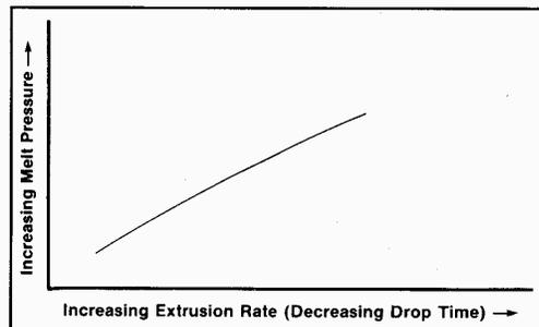
**Fig. 1: Melt Flow as Expected**
