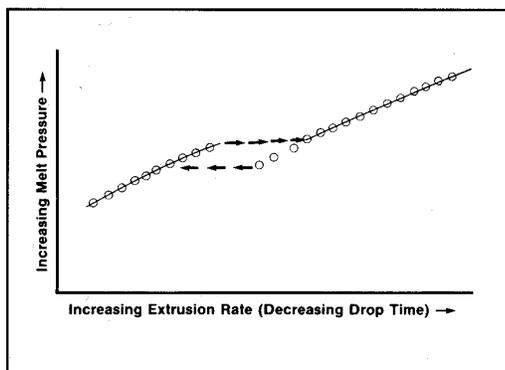
**Fig. 3: Pressure and Extrusion Rate Oscillations in the Pressure Plateau Regions Produce Sharkskin**
